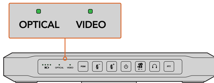
When a valid video signal is detected via SDI or HDMI, you'll see ATEM Camera Converter's 'video' status indicator illuminated. The 'optical' indicator will illuminate when a valid SDI signal is detected via the optical fiber input.
