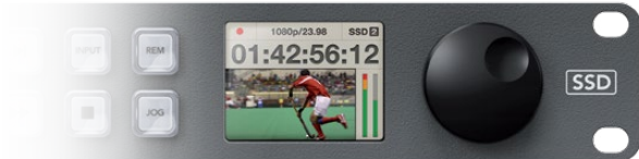
HyperDeck Studio shows embedded SDI timecode on its display.
