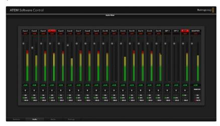
ATEM switchers include a built-in audio mixer that lets you use the embedded HDMI and SDI audio from your cameras, media servers and other inputs without the need for an external audio mixer. This is perfect when using an ATEM switcher on location or in small spaces within modern OB vehicles as you don't have to find room for an external audio mixer. The audio is mixed in the Audio tab of ATEM Software Control and output over the SDI and HDMI program outputs.
