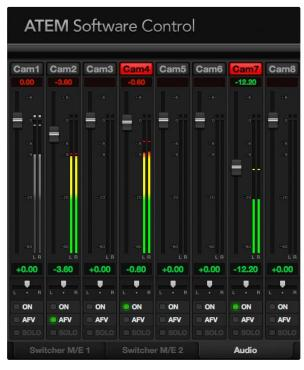
Step 4: Try sliding the gain faders up and down on your hardware control surface and verify that the audio mixer faders show a corresponding increase and decrease in the software on your computer screen.
