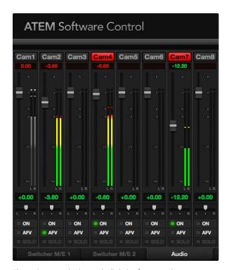
The audio mixer displays red tally lights for any audio sources that are currently on air, as well as audio level, audio balance and checkboxes for selecting which audio should be used.
