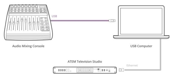
You can adjust multiple audio levels at the same time by connecting a hardware audio mixer to the computer which is running ATEM Software Control.
